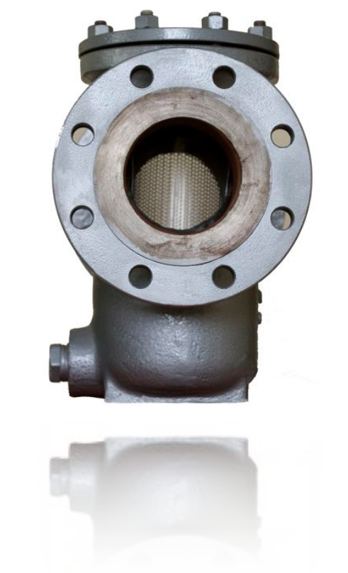
4" CLASS 150 BOLTED BASKET FLANGED WCB - SIDE VIEW
